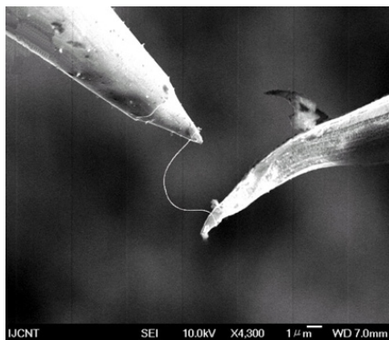
Fig. 8. Bending of a single Carbon Nanotube.
