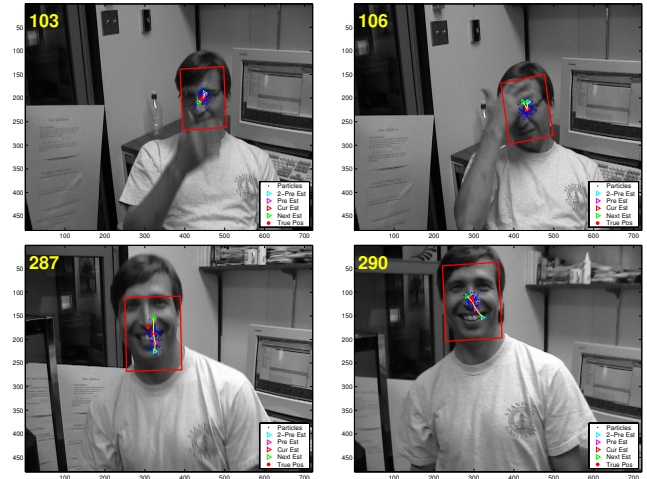
Fig. 5. Tracking results of our approach. In this experiment, we use 100 particles in every frames, and achieve 20 frames/sec on our 3.0GHz PC.
