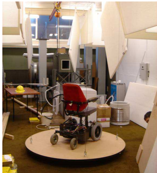
Fig. 8. Quadrifilar Pendulum setup for moment of inertia
