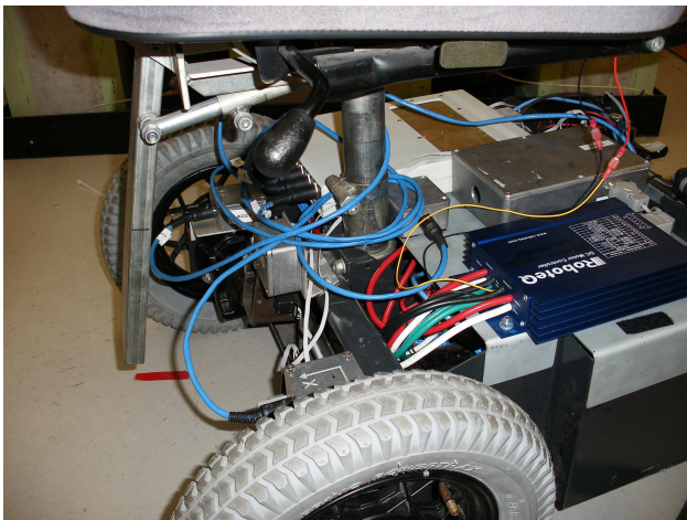
Fig. 3. RoboteQ Controller and battery connections.
