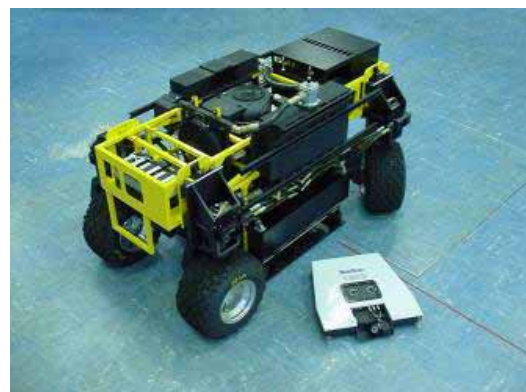
Fig. 25. Marsupial parking lot surveillance system.
