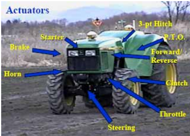
Fig. 26. Actuators used to retrofit a tractor.
