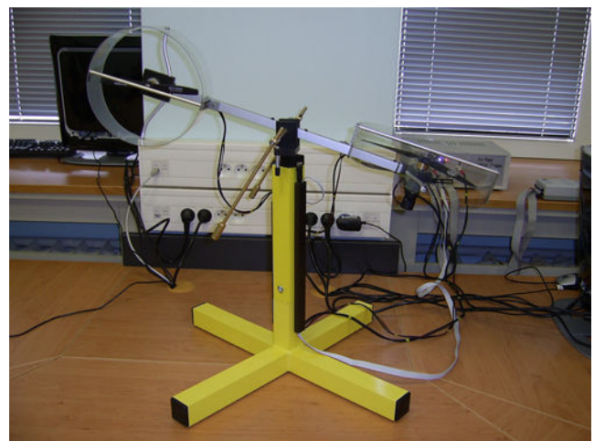
Fig. 1. Two-rotor aerodynamic system
