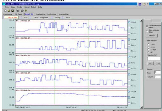
Figure 2. MV/DV plots during the plant test.
