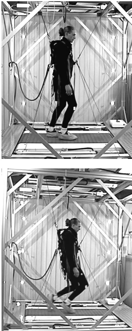
Fig. 5. Robot STRING-MAN: Robot with seven strings (above); Virtual safety corset for testing balance (below).
