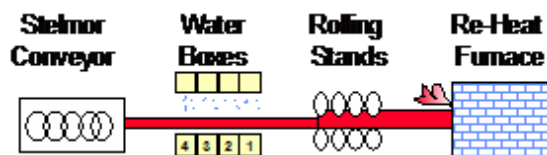
Fig. 4. Bar steel mill process diagram
