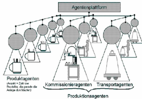
Fig. 7. Fully distributed agent-based architecture
