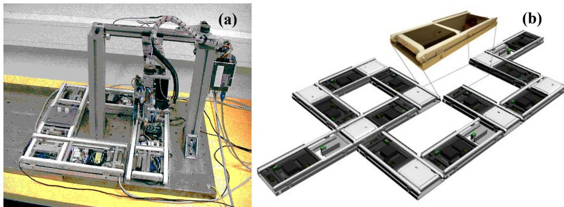
Fig. 6. (a) ABAS pilot installation in a micro-assembly cell (b) Actor-based transporter
