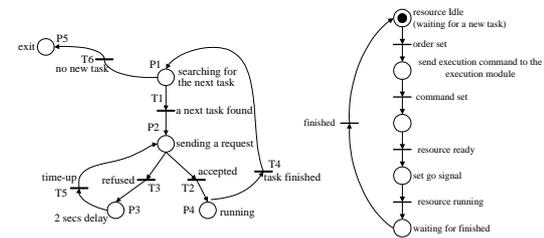
**Figure 3 Petri-net model of a resource holon (left) and a product holon (right)**
