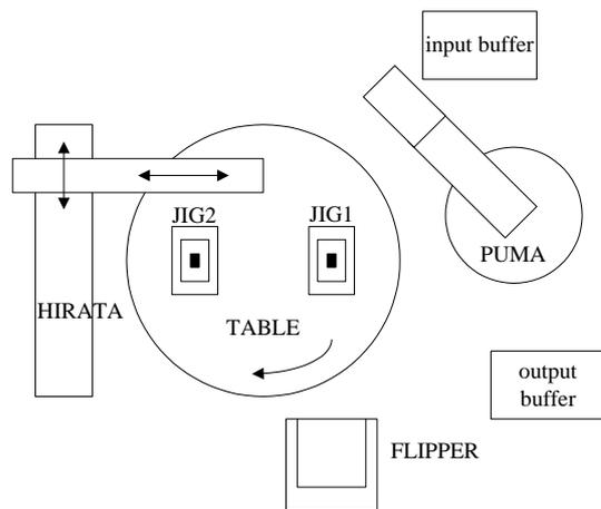
Figure 1 Layout Of The Robot Assembly Cell
