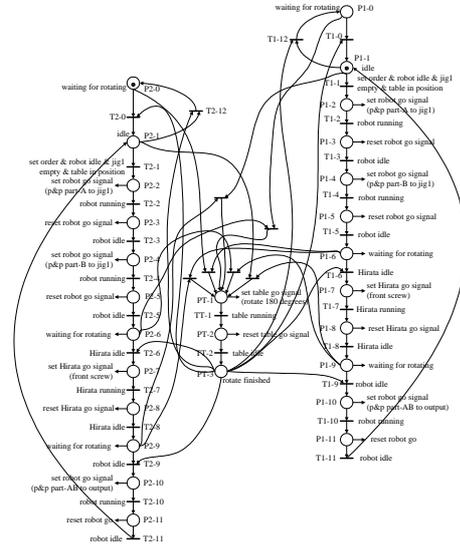
**Figure 2. Petri-net model of a conventional approach for Scenario I**
