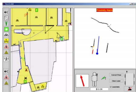
Fig. 9. Human interface with map including the navigated route (left) and real-time scanner data with proximity alarm (right).
