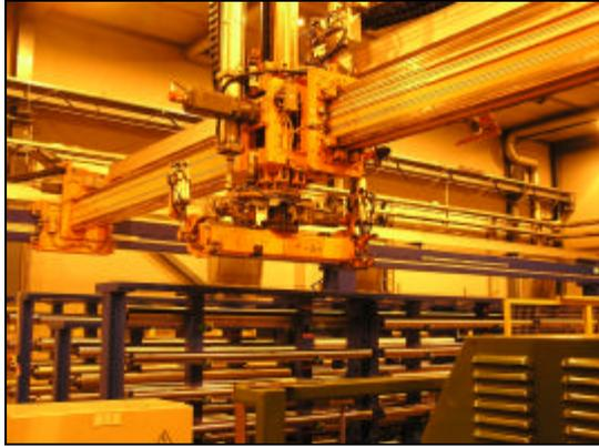
Fig. 7. The SZ-roll storage crane.
