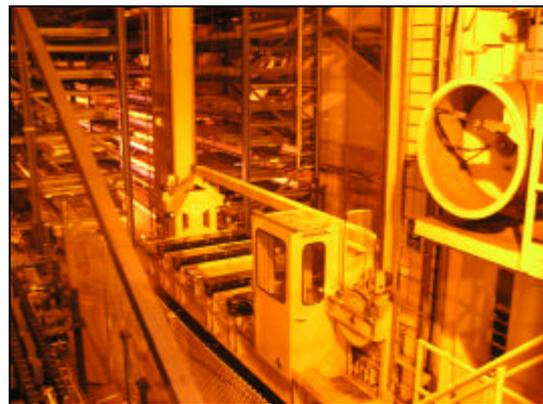
Fig. 6. Automatic high bay storage crane
