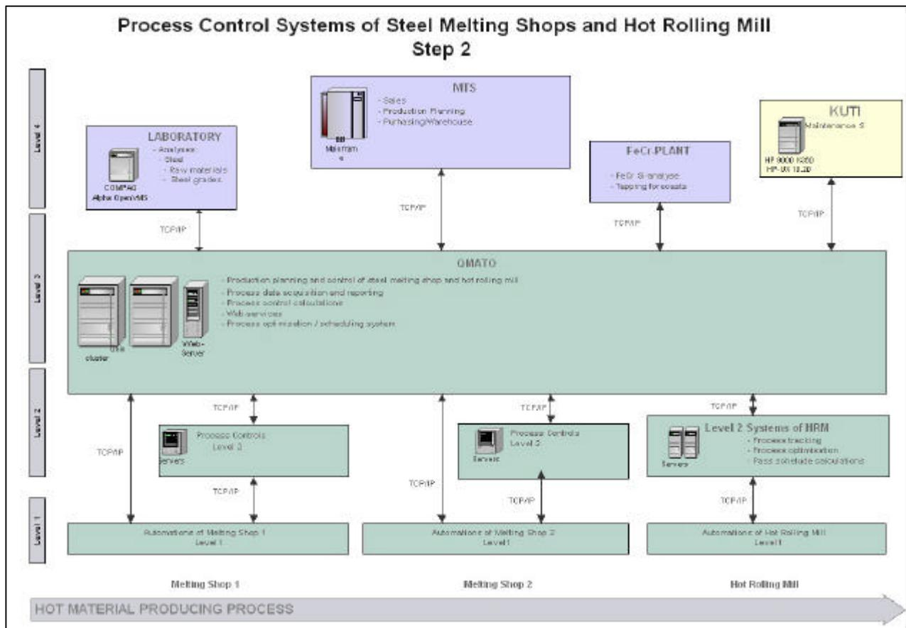
Fig. 1. Example of automation levels in Steel Melting Shops and Hot Rolling Mill
