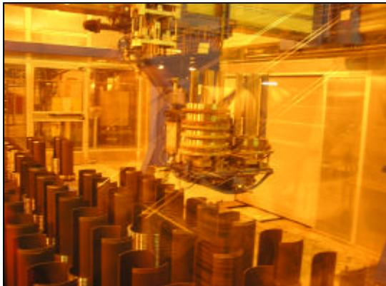
Fig. 8. The slitting tool assembly robot.
