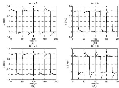
Fig. 3. The command tracking performance of the backstepping controller for the aerodynamic uncertainties. (a)  $A + \Delta A$ , (b)  $A - \Delta A$ , (c)  $B + \Delta B$  and (d)  $B - \Delta B$  (solid: adaptation rule, dash: non-adaptation rule)
