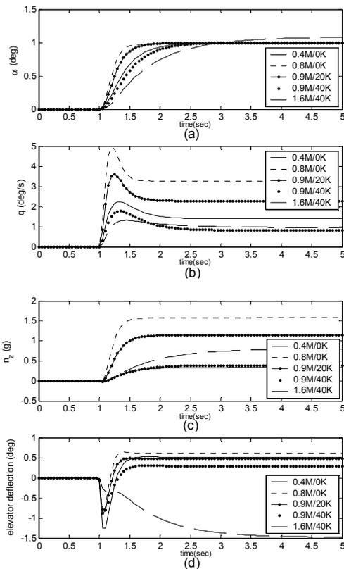
Fig. 2. Step responses of backstepping controller. (a) Angle-of-attack, (b) pitch rate, (c) normal acceleration and (d) surface deflection.
