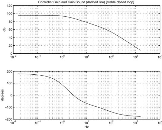
Fig. 9. The controller gain and phase (solid lines) and the gain bound (dashed line) due to actuator limitation.
