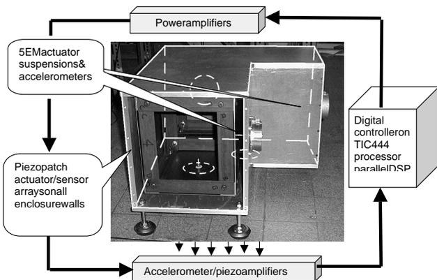
Fig. 1. Enclosure control setup.
