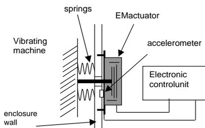
Fig. 2. Electronically controlled suspensions.
