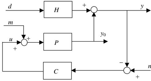
Fig. 7. Block diagram of the active mount feedback system for vibration isolation.
