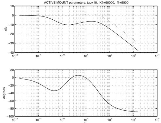
Fig. 8. Bode plots of the vibration isolation dynamics of the passive mount (dashed lines) and the active mount (solid lines).
