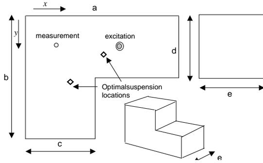
Fig. 4. An excitation point and a measurement point on an L shaped plate of the enclosure.
