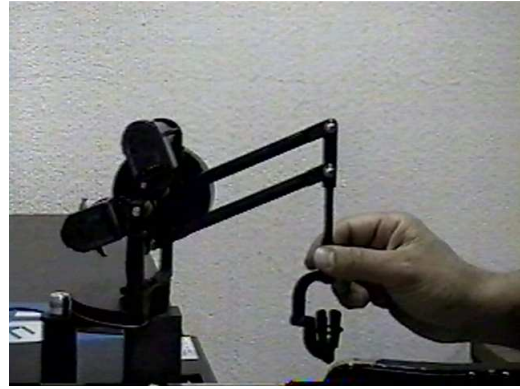
Figure 2. Gripping the haptic device with three fingers in order to reduce degrees of freedom.
