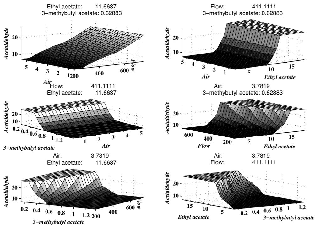
Fig. 7. Model surfaces of a five variable LE model on a normal operating point.
