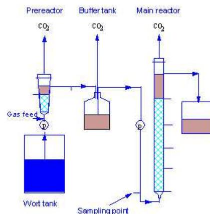
Fig. 2. Pilot scale continuous fermentation system.
