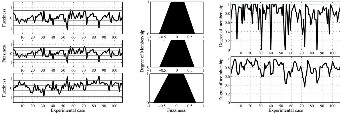
Fig. 8. Detection of operating conditions with LE models: fuzziness and limits of fuzziness for three equations and the resulting degrees of membership for each data point (upper curve) and a moving average (lower curve).
