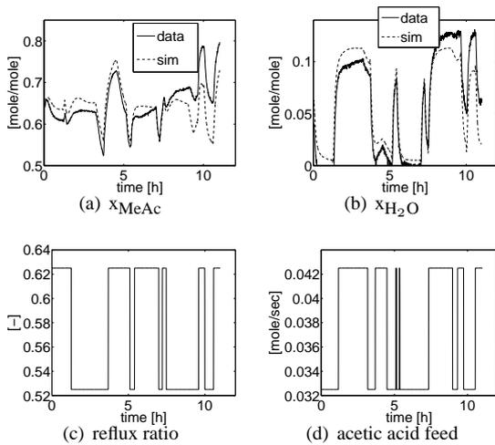
Fig. 4. Identification data (data) and the corresponding simulated outputs of the reduced-order linear model (sim).
