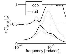
Fig. 8. Robustness constraints with optimal control performance controller (ocp) and reduced-order PI controller (red).
