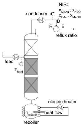
Fig. 2. Scheme of the semibatch reactive distillation column.
