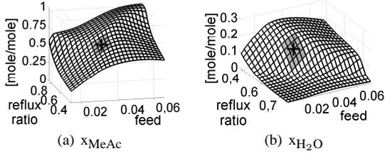
Fig. 3. Stationary characteristic diagrams of the CVs (heat flow = 3.667 kW).
