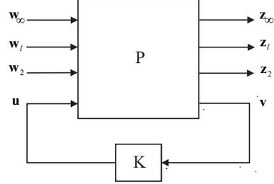
Fig. 1. Generalised plant configuration for multiobjective performance calculation.
