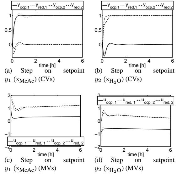
Fig. 7. Closed-loop step responses with optimal control performance controller (ocp) and reduced-order PI controller (red), all variables scaled according to (18).
