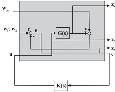
Fig. 6. Generalised plant for multiobjective design.
