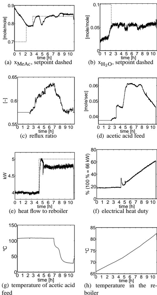
Fig. 9. Experimental results in a setpoint and disturbance rejection scenario.
