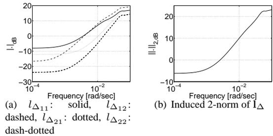
Fig. 5. Output-multiplicative uncertainty as a result of the identification scheme.
