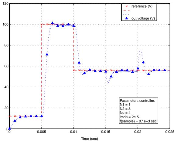
Fig. 2. Reference and output voltage response.
