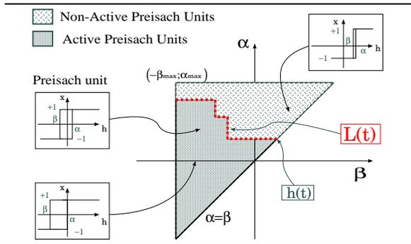
Fig. 3. Preisach units for different threshold parameters  $(\alpha, \beta)$ .
