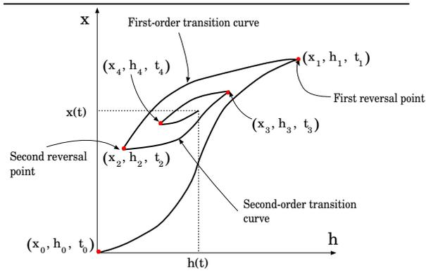
Fig. 2. An example of hysteresis multi-branching nonlinearity. Hysteresis branches are also called transition curves.
