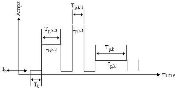
Fig. 1. Keyhole-Plasma Welding Process.
