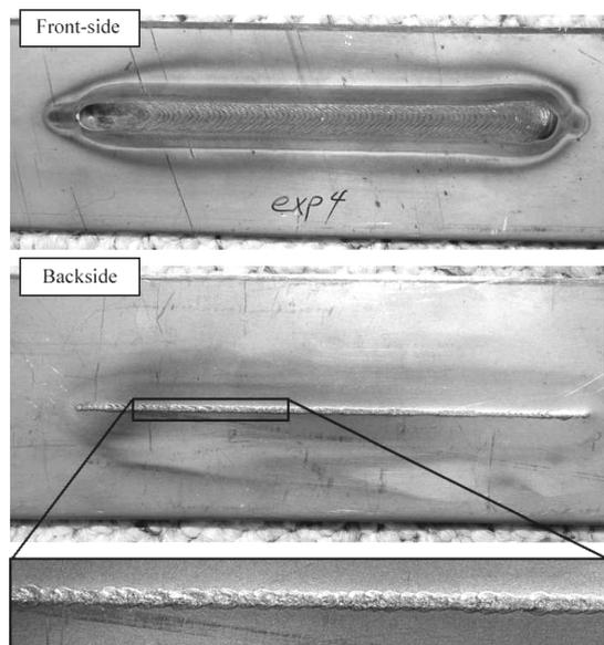
Fig. 5. Weld Images (Front View, Backside View, and Zoomed View of Backside)
