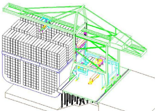
Fig. 2. Schematic configuration of high efficiency gantry crane system.
