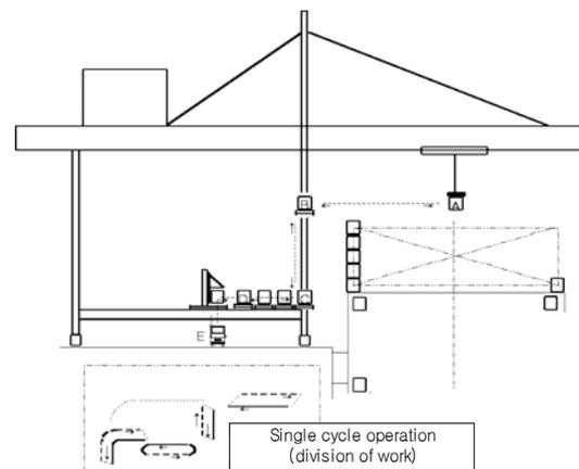
Fig. 3. Operation structure of single cycle crane system.
