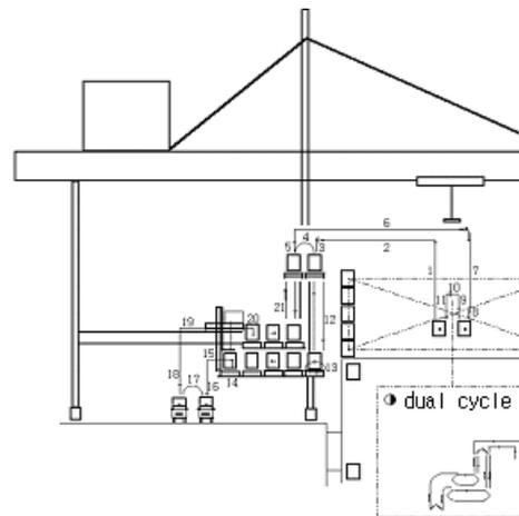
Fig. 5. Operation process of new type crane system. (dual cycle)
