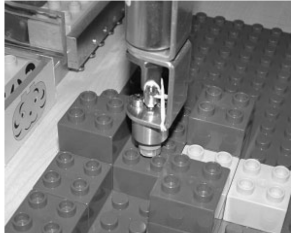
Fig. 2. Inserting of a new brick despite of the “crowded” surrounding
