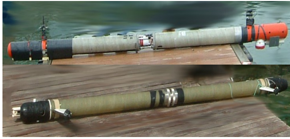
Fig. 1. The first (top) and second (bottom) version of the Følaga. The main difference between the two versions is in the vertical propulsion pumps: in the first version there is one pump placed at the center of the vehicle, in the second version there are two pumps placed at the bow and stern of the vehicle respectively.
