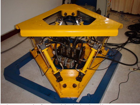
Fig. 1. Stewart platform with six hydraulic actuators
