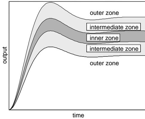
Fig. 1. Three zones defined by error-bounded envelopes
