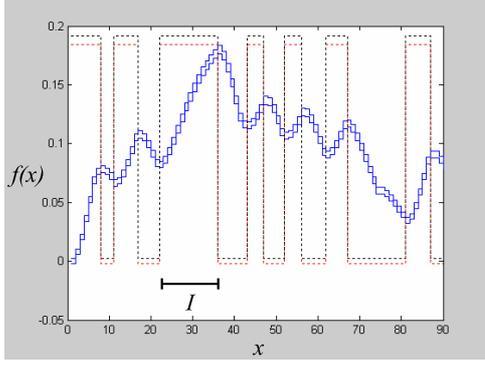
Fig. 3. Monotony analysis from measurement.  $f(x)$  is the measurement,  $x$  is the step time and  $I$  is the interval of monotony.
