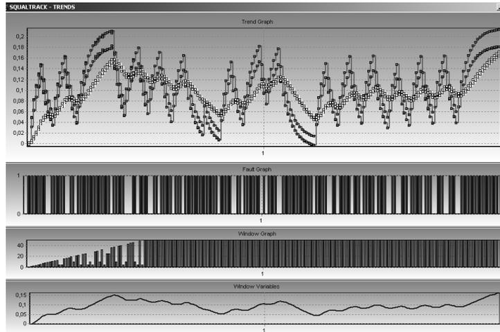
Fig. 4. SQualTrack fault detection. Case 2: J-bigger. Upper graph shows envelopes of measurement and simulation. Following graph shows bars with 1 when a fault is detected. Next graph indicates last window length applied at the specific time. Lower graph shows the analyzed measurement.
