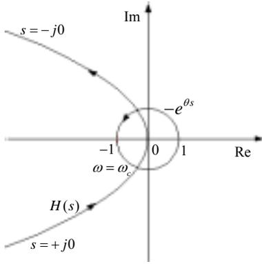
Fig. 4. The loci of  $H(s)$  in(18) and  $-e^{j\omega\theta}$
