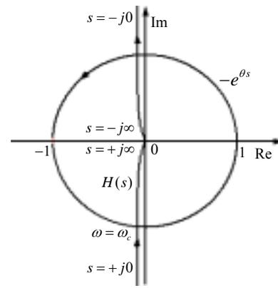
Fig. 2 The loci of  $H(s)$  in (8) and  $-e^{j\omega\theta}$
