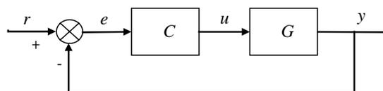
Fig. 1. Feedback control system equation
