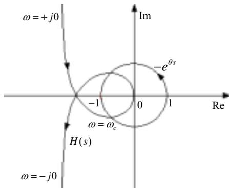
Fig. 5. The loci of  $H(s)$  in (28) and  $-e^{j\omega\theta}$
