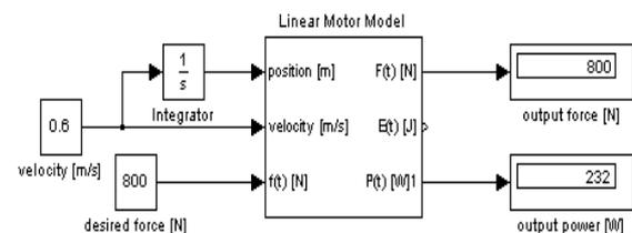
Fig. 5. Linear motor input-output model.
