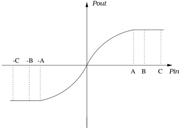
Fig. 1. Typical transfer property of a RF PA.  $[-A, A]$  is a weakly nonlinear area,  $[-B, B]$  is slightly into saturation and  $[-C, C]$  is largely saturated.
