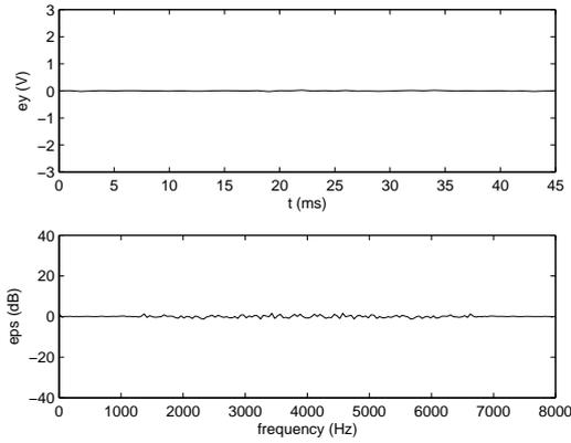
Fig. 4. The estimation errors in both the time and frequency domains given by the infinite VS model.
