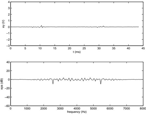
Fig. 8. The estimation errors in both the time and frequency domains given by the finite VS model.
