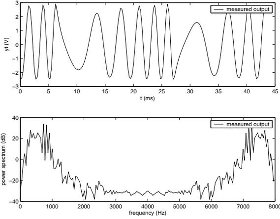
Fig. 3. The measured time series and frequency response when the PA works in  $[-A, A]$ .
