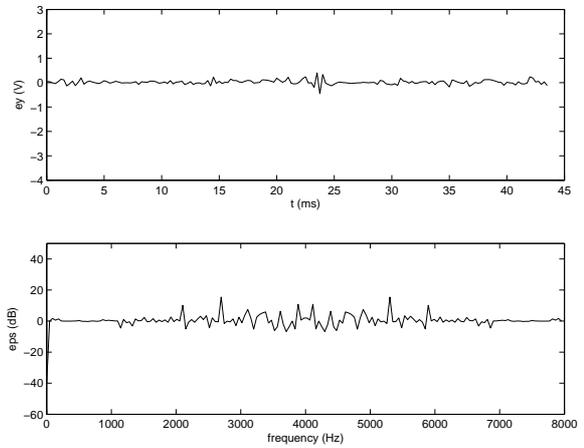
Fig. 11. The estimation errors in both the time and frequency domains given by the finite VS model.
