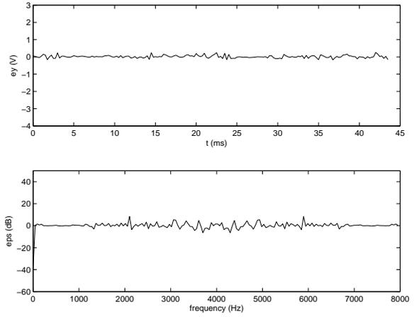
Fig. 10. The estimation errors in both the time and frequency domains given by the infinite VS model.
