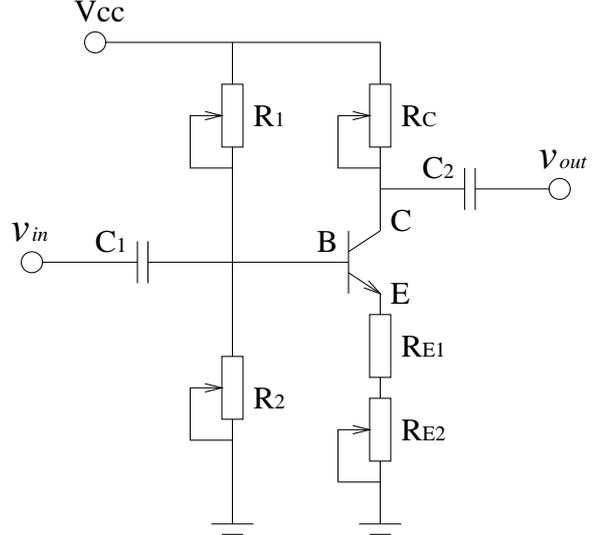
Fig. 2. Amplifier circuit with  $R_1 = 370\Omega$ ,  $R_2 = 430\Omega$ ,  $R_C = 198\Omega$ ,  $R_{E1} = 18\Omega$ ,  $R_{E2} = 19\Omega$  and  $C_1 = C_2 = 0.1\text{mf}$ . The NPN epitaxial silicon transistor is BC546 from FAIRCHILD SEMICONDUCTOR®.
