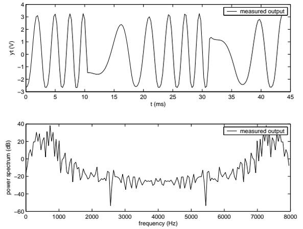
Fig. 6. The measured time series and frequency response when the PA works in  $[-B, B]$ .
