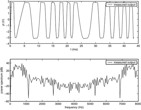
Fig. 9. The measured time series and frequency response when the PA works in  $[-C, C]$ .
