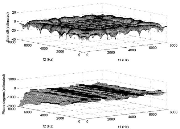
Fig. 12. Predicted second order frequency response given by the infinite VS model.
