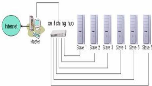
Fig. 1. Construction diagram of PC cluster system
