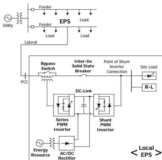
Fig. 1. Configuration of the PPS
