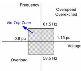
Fig. 4. Window-relaying method
