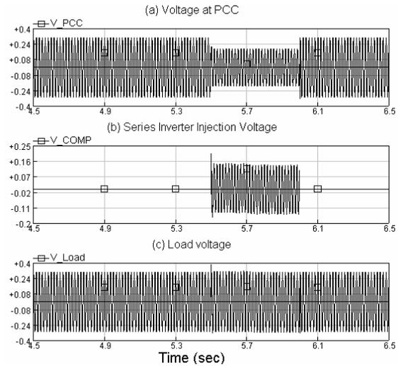
Fig. 7. Simulation result: voltages
