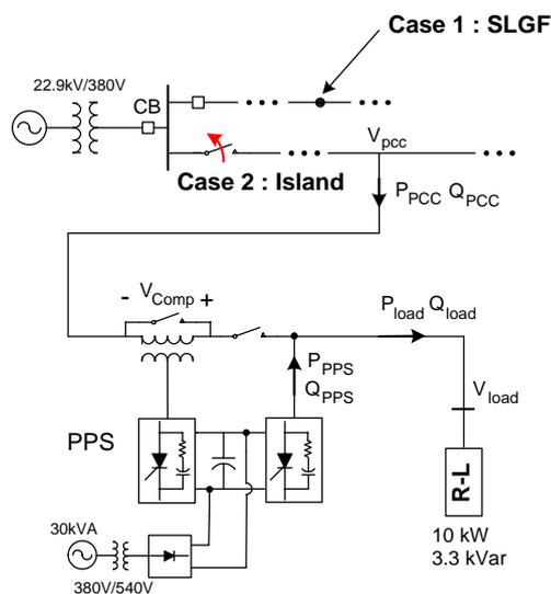
Fig. 5. Distribution system for simulation
