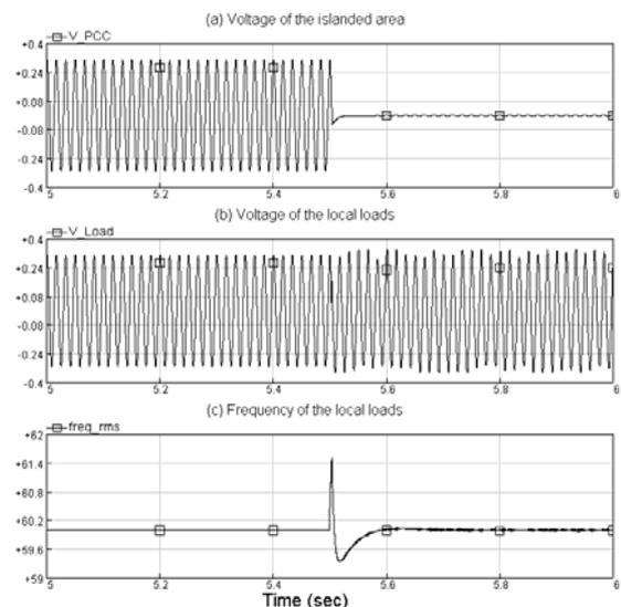
Fig. 8. Simulation result: voltage and frequency
