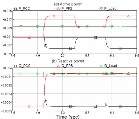
Fig. 6. Simulation result: active and reactive power
