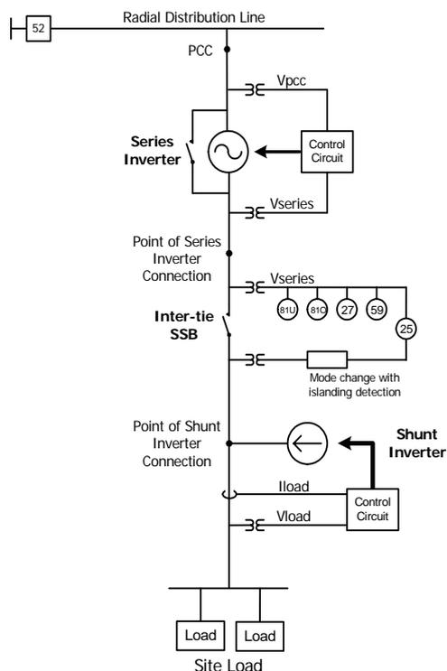
Fig. 3. Configuration of control circuits of the inverters and the inter-tie SSB
