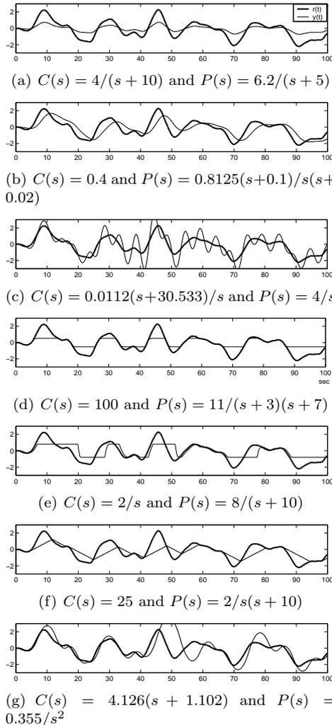
Fig. 3. Track loss in system of Figure 1(a)
