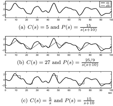
Fig. 2. Tracking of random reference in system of Figure 1(a)
