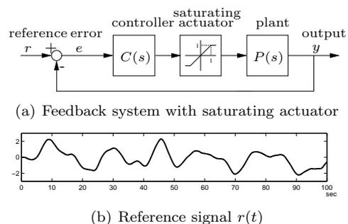
Fig. 1. Feedback control system with saturating actuator and reference signal
