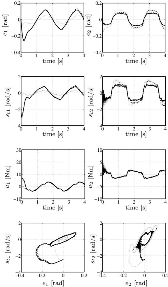
Fig. 4. Experimental Result (solid:  $T = 0.05$  [s], dashed:  $T = 0.1$  [s], dot-dashed:  $T = 0.3$  [s]), dot: Inverse optimal control)
