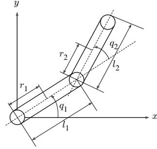
Fig. 2. Schematic diagram of the two-link direct drive manipulator
