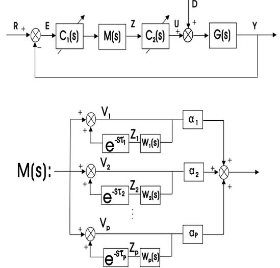
Fig. 1. Non-linear adaptive MIMO multi-periodic repetitive control system
