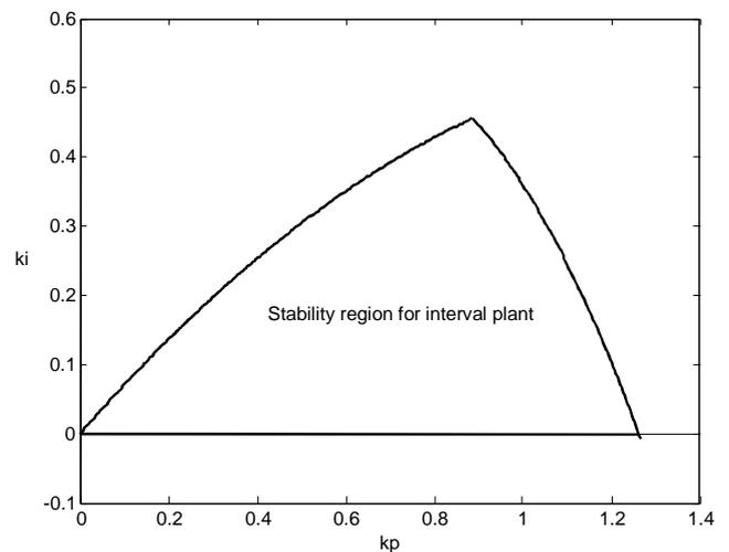
Fig. 9: Stability region for interval plant of motor
