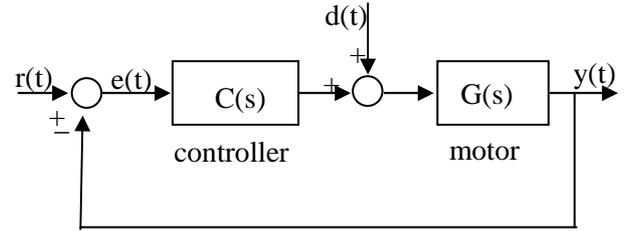
Fig. 7: Position control system
