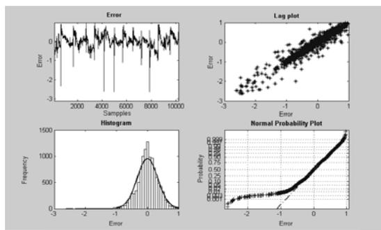
Fig. 3: 4- plot of the residual of the linear model (residual trend, histogram, normal probability plot and its dispersion).
