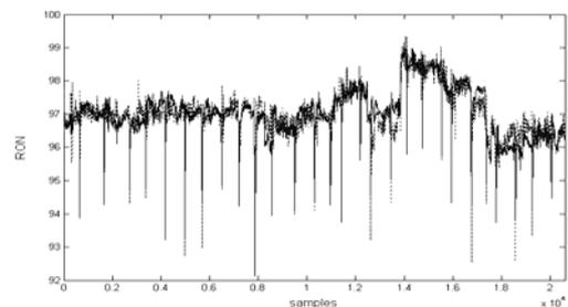
Fig. 10: Acquired RON values (dotted line) and their nonlinear estimation (solid line) – scaled units, two working points.
