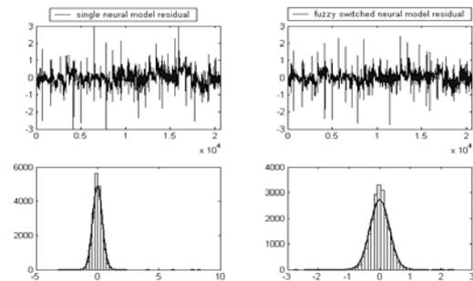
Fig. 13: On-line behaviour of the single neural model and the fuzzy switched model: residual trends and histograms.
