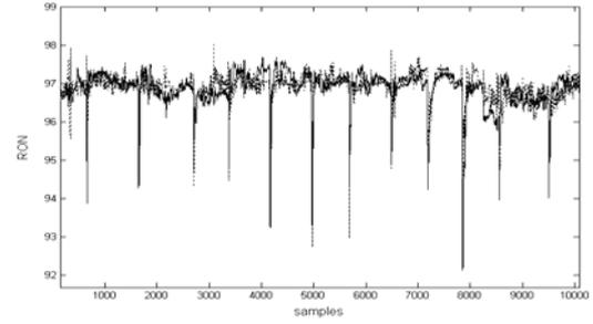
Fig. 7: Acquired RON values (dotted line) and their nonlinear estimation (solid line) – scaled units, one working point.
