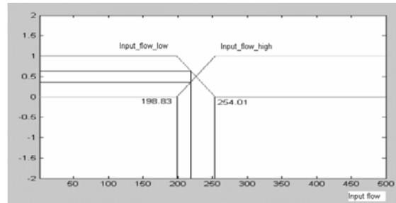
Fig. 9: membership functions for the variable *input\_flow* - scaled values
