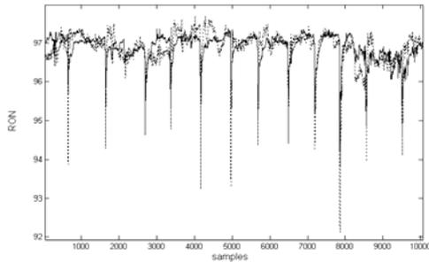
Fig. 2: Acquired RON values (dotted line) and their linear estimation (solid line) – scaled units
