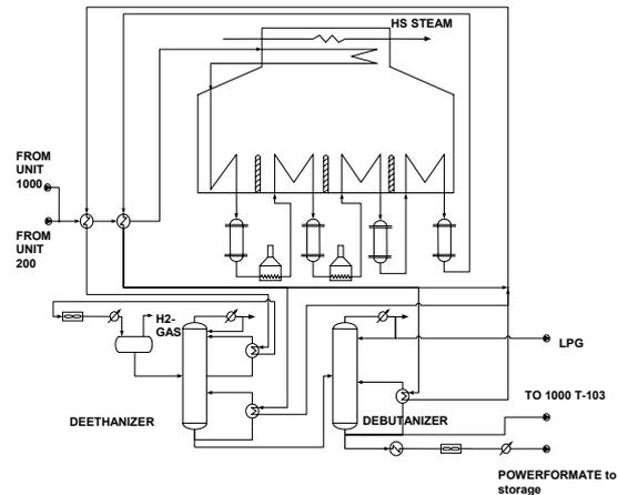
Fig. 1 The Powerformer Unit
