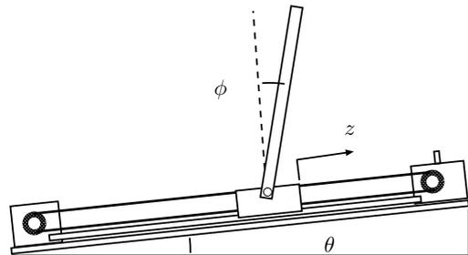
Fig. 7. Inverted pendulum system on a slope
