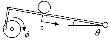
Fig. 3. Ball & Beam System
