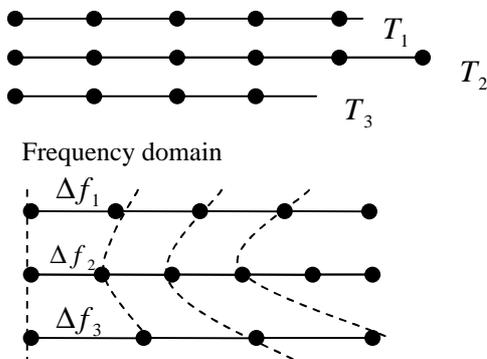
Fig. 2 Multiple revolution data without interpolation in the time and frequency domains
