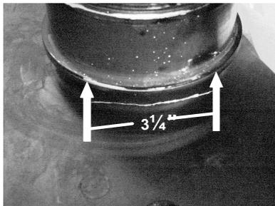
Fig. 5 Planetary Carrier Plate with a Crack
