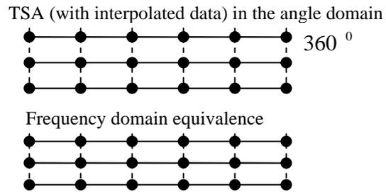
Fig. 3 TSA data samples in the angle domain and the corresponding frequency domain
