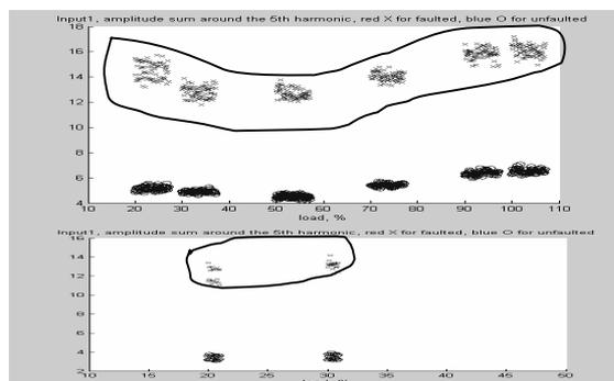
Fig. 6 Harmonic Index around the 5th harmonic of Input1 in test cell and on-aircraft
