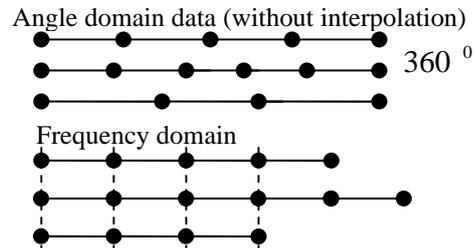
Fig. 4 Multiple revolution data without interpolation in the angle and frequency domains
