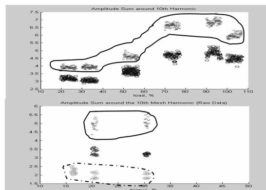
Fig. 7 Harmonic Index around the 10th harmonic of PortRing in test cell and on-aircraft
