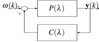
Fig. 1. Closed-loop System
