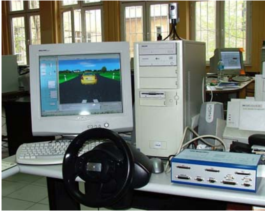
Fig. 3. Human-in-the-loop simulation setup
