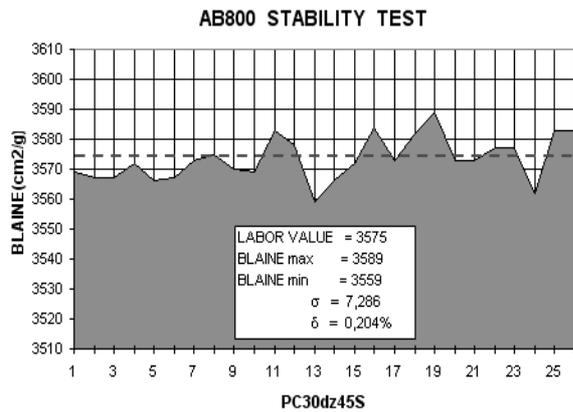
Fig. 3. Stability test results of the AB800
