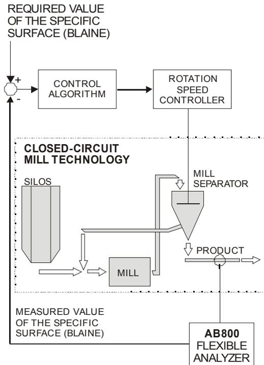
Fig. 1. Principal scheme of the AB800 analyser utilization in the process
