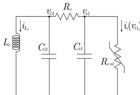
Fig. 2. Generator of the reference voltage
