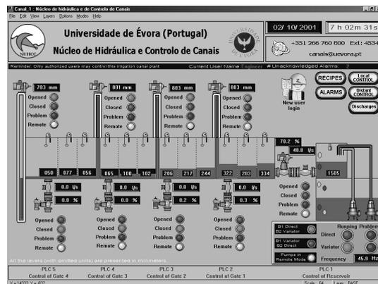
Fig. 12 – SCADA application (main menu)
