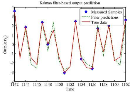
Fig. 4. Comparison of Kalman filter predictions with true output in the underdamped system
