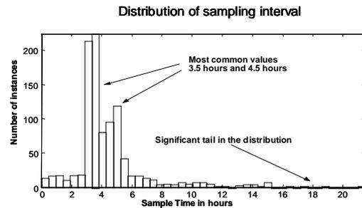
Fig. 6. Distribution of the output sampling intervals
