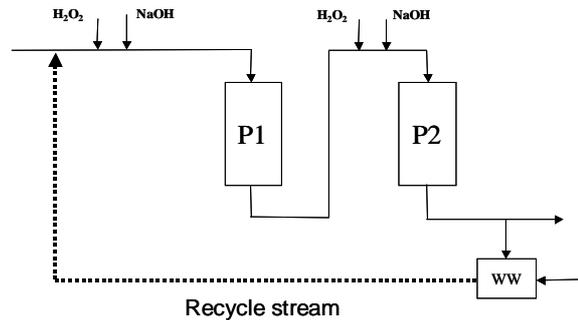
Fig. 5. Simplified flow sheet of Mechanical Pulp mill
