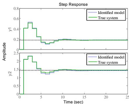
Fig. 3. Comparison of step responses of the underdamped system
