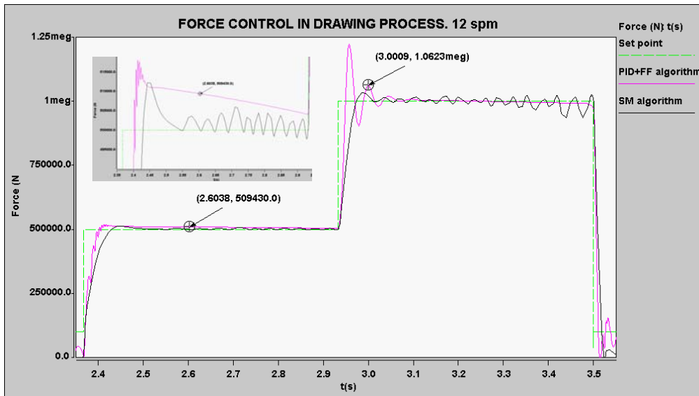
Fig. 6. Results in simulation with FF based algorithm and sliding mode algorithm at a rate of 12 spm.
