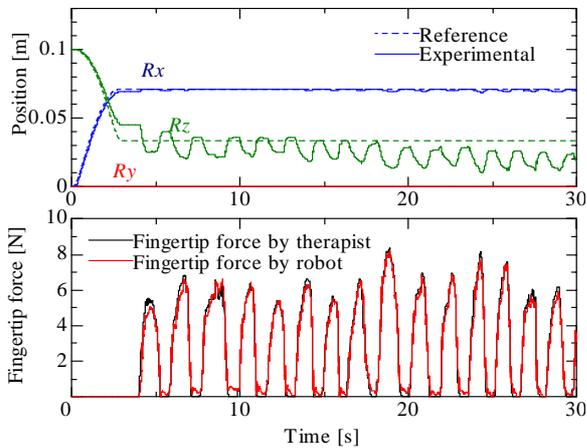
Fig.10 Experimental results of the 4<sup>nd</sup> finger for massage control
