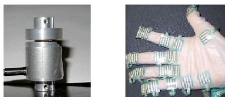
(a) 6-axis force sensor (b) Sheet-type glove sensor
