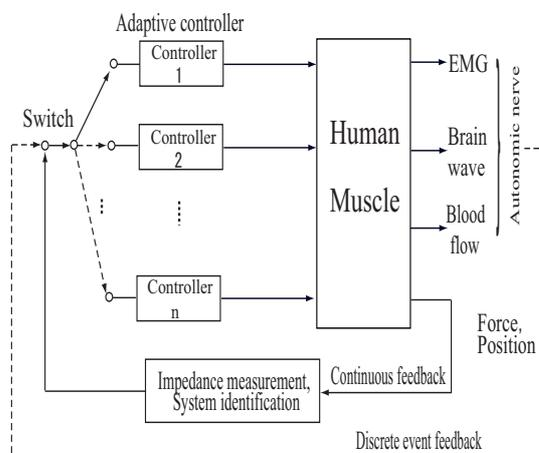
Fig.12 Autonomous sense feedback control system of Human muscle for relaxation of human body and heart
