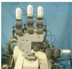
Fig.1 TUT hand with 6-axis force sensor
