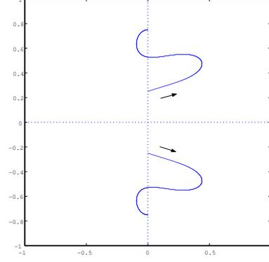
Fig.1. Conjugate pole loci of true time-varying system.
