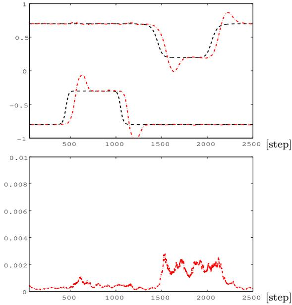
Fig.6. Sample mean (top) and variance (bottom) of the real part of predicted sudden change system ( $N = 100$ ,  $L = 50$  (50-step ahead prediction)).
