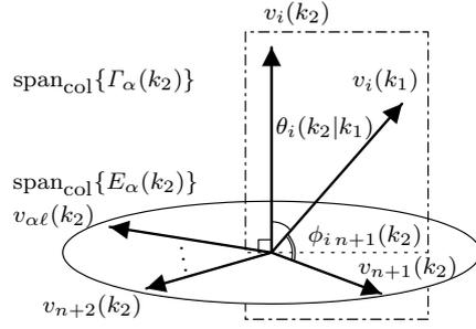
Fig.A.1. Relation between signal and noise subspaces.
