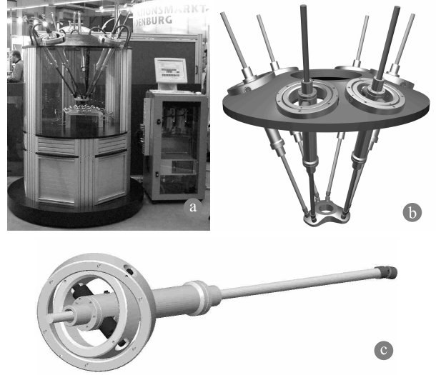
Fig. 4. PKM PaLiDA - a: Test bed at the Hannover Industrial Fair 2001, b: CAD-model, c: single strut with integrated linear direct drive
