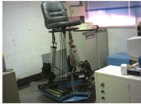
Fig. 1 The experimental parallel manipulator
