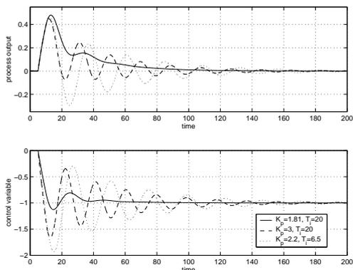
Fig. 3. Example of a load disturbance response for a too high value of  $T_i$  (solid line), for too high values of  $K_p$  and  $T_i$  (dashed line) and for too high value of  $K_p$  and a too low value of  $T_i$  (dotted line).
