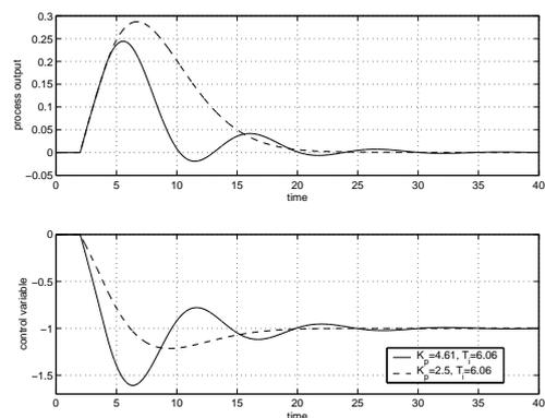
Fig. 4. Load disturbance responses for  $P_1(s)$  with  $K_p = 4.61$  and  $T_i = 6.06$  (solid line) and with  $K_p = 2.5$  and  $T_i = 6.06$  (dashed line).
