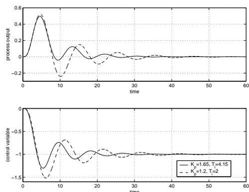
Fig. 5. Load disturbance response for  $P_2(s)$  with  $K_p = 1.65$  and  $T_i = 4.15$  (solid line) and with  $K_p = 1.2$  and  $T_i = 2$  (dashed line).
