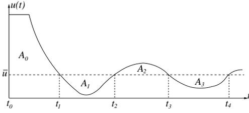
Fig. 1. Significant parameters for determining the Area Index.
