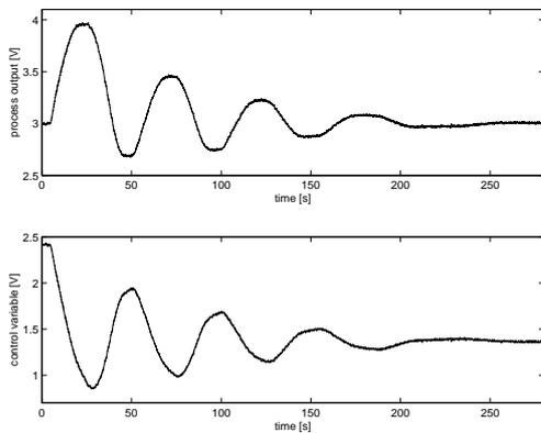
Fig. 7. Experimental load disturbance response with  $K_p = 1$  and  $T_i = 25$ .
