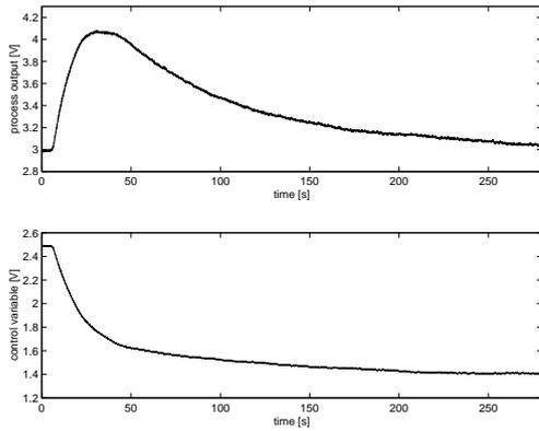
Fig. 6. Experimental load disturbance response with  $K_p = 0.5$  and  $T_i = 50$ .
