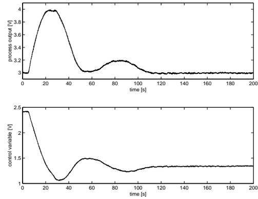
Fig. 8. Experimental load disturbance response with  $K_p = 0.8$  and  $T_i = 25$ .
