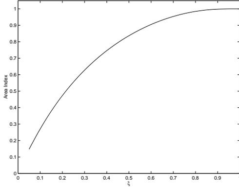
Fig. 2. Dependence of the Area Index from the damping factor  $\xi$ .
