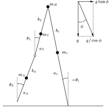
Fig. 15. Parameters of Walking Machine (Yamakita and Asano)
