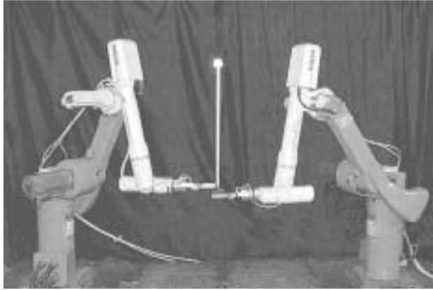
Fig. 8. Transfer of Pendulum
