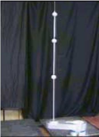
Fig. 7. Triple Spherical Pendulum
